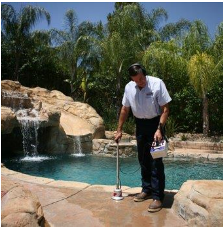
Figure 18: Acoustic leak detection
